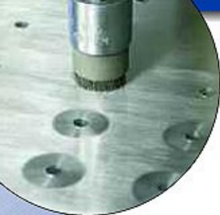
Cleaning around rivet holes on an aluminum aircraft panel.
