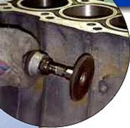
Deflashing a cast iron engine block.
