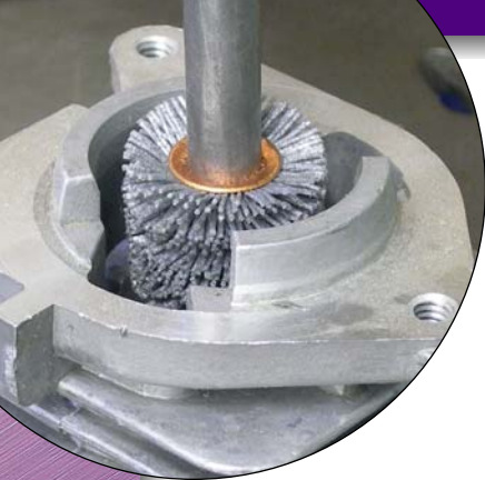
Deburring the internal bores of an air-cooled cylinder head.
