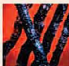
A microscopic view shows abrasive grain impregnated Nylox filaments.
