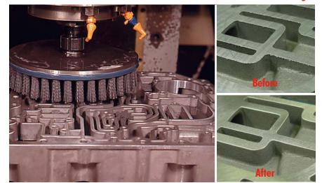
Problem: Burrs on transmission components can break away from parent components during use and cause transmission wear and eventual failure. Therefore, fluid passages must be completely burr-free.
