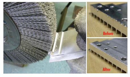
Problem: Computer and communications equipment contain aluminum heat sinks which are critical to dissipate the heat produced by these systems. Machined surfaces on heat sinks ensure tight fit and proper mounting characteristics. However, burrs produced by machining processes must be removed to ensure they do not fall into the electrical components and short circuit their operation.
