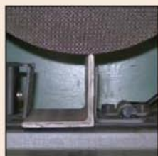
Incorrect (Wide contact point)
