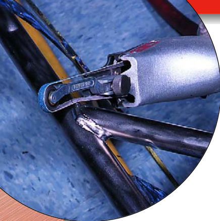
Blending a weld using a portable file belt.
